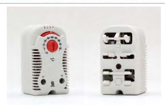
The TTEC series are thermostat controllers used to regulate the temperature inside industrial control panels or cabinets and control cabinet accessories. The TTEC series, bimetallic thermostats, control fans, heaters, and switch loads. TTEC-100 and TTEC-200 are identical except the TTEC-100 is Normally Closed which opens at temperature rise, the TTEC-200 is Normally Open which closes at temperature rise. Both are available in Fahrenheit or Celsius
